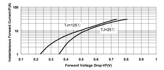
Fig.3-Typical Instantaneous Forward Voltage Characteristics
