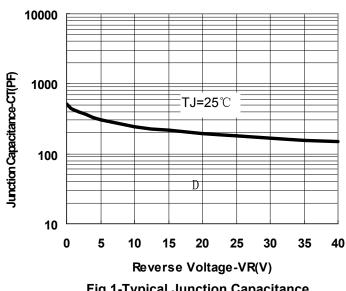
Fig.1-Typical Junction Capacitance
