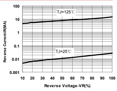
Fig.2-Typical Reverse Characteristics
